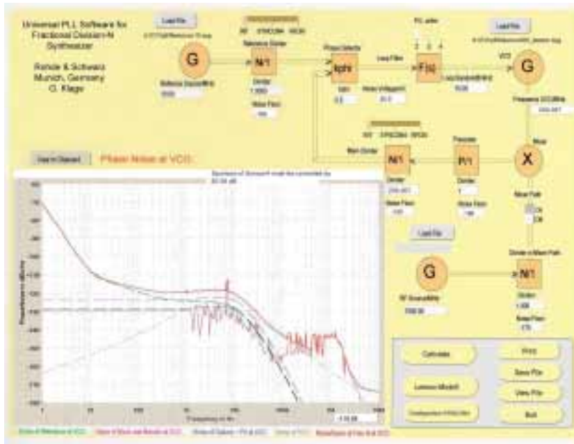
Figure 25. Universal synthesizer software screen image with the various contributions as explained in the above text. It can handle single loop synthesizers multi-loop synthesizers, including up multiplication ( N < 1 ) and marked as divider in mixer path. Finally, it also allows to calculate the spurious contents using the fractional synthesizer principle based on the digital compensation scheme. This is done in a separate portion of the software.
